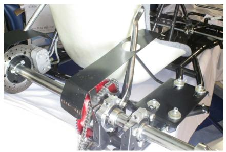
**Sprocket Guard** 1 piece \*FIT KIT not included – you should not require any additional bolts if a seat and axle is already fitted to your chassis.
