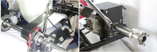
Seat Stays 2 pieces \*FIT KIT – if a seat is already fitted to your chassis with only 4 points, you will need another 2 points worth of bolts to fit this item. You will need 2x M8x35-50mm bolts (depending on whether you use nylon spacers and large OD washers), 2x 8mm Nylon seat Spacers (optional), 2x M8 Nyloc Nuts, 2x M8 Machine Washers, 2x 35mm OD / 8mm ID countersunk seat washers, 2x large OD flat seat re-inforcement washers (optional).
