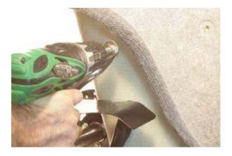
d. Fit a bolt through one of the 35mm OD / 8mm ID countersunk seat washers, then through the seat hole you just drilled, then through the large OD seat washer, then through one of the 8mm Nylon Seat spacers, then through the top of the seat stay, then through an M8 machine washer and finally fix in place with an M8 Nyloc Nut.
